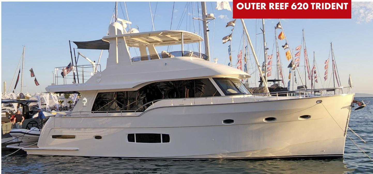
**The Outer Reef 620 Trident is a Ward Setzer design with excellent cruising qualities from 8 to 24 knots and long range capabilities. In addition, the yacht's hard top is designed to hydraulically lower to allow for bridge clearances while cruising. Other Trident models include the 720, 980, and 106 models.**
